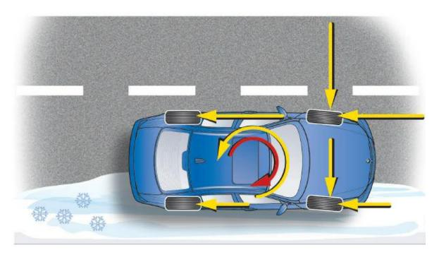
This active counter-steering creates counter-torque about the z or vertical axis (red arrow) which compensates for the earlier acting yawing force (yellow arrow).
